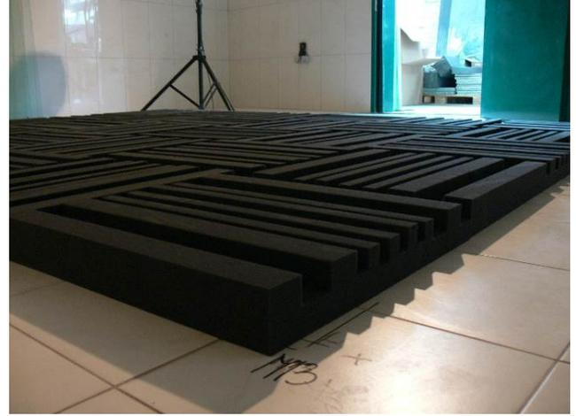
Picture 6: exposed perimeter edge of test samples.
