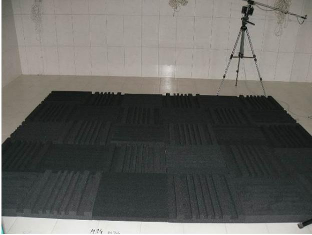
Picture 5: test samples in the reverberation room.
